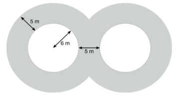
2.19.2 Competition Vehicles must be able to negotiate a slalom course in less than 11.5 seconds, in all driving configurations.
