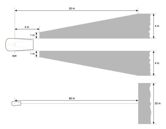
2.17.2 Rear vision systems may be electronic, mirrors, or both. Rear vision systems must operate whenever the Competition Vehicle is in motion under its own power or about to be driven. Rear vision images must be upright and oriented so that objects on the right of the Competition Vehicle are on the right of the image.
